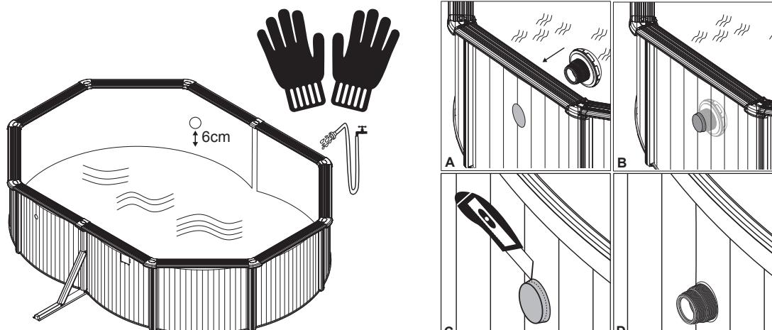
**NOTE:** Before connecting valve to the pool, fill the pool leaving 5 - 6cm of space between the position of the connection valve and water surface.
