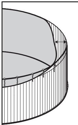
**NOTE:** The liner of the steel wall pool is designed to be smaller than the steel wall for technical reasons. If you find it difficult to assemble the liner, place the liner under the sun for one hour which will make it more pliable. You should then be able to assemble the liner step by step, stretching it by hand at the same time. This procedure will not damage the liner.
